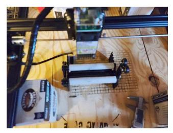
Center the YRR under the laser in the middle of your bed, with the stepper motor on the left side, aligning it **parallel to the X-Axis** as shown in the image above.
